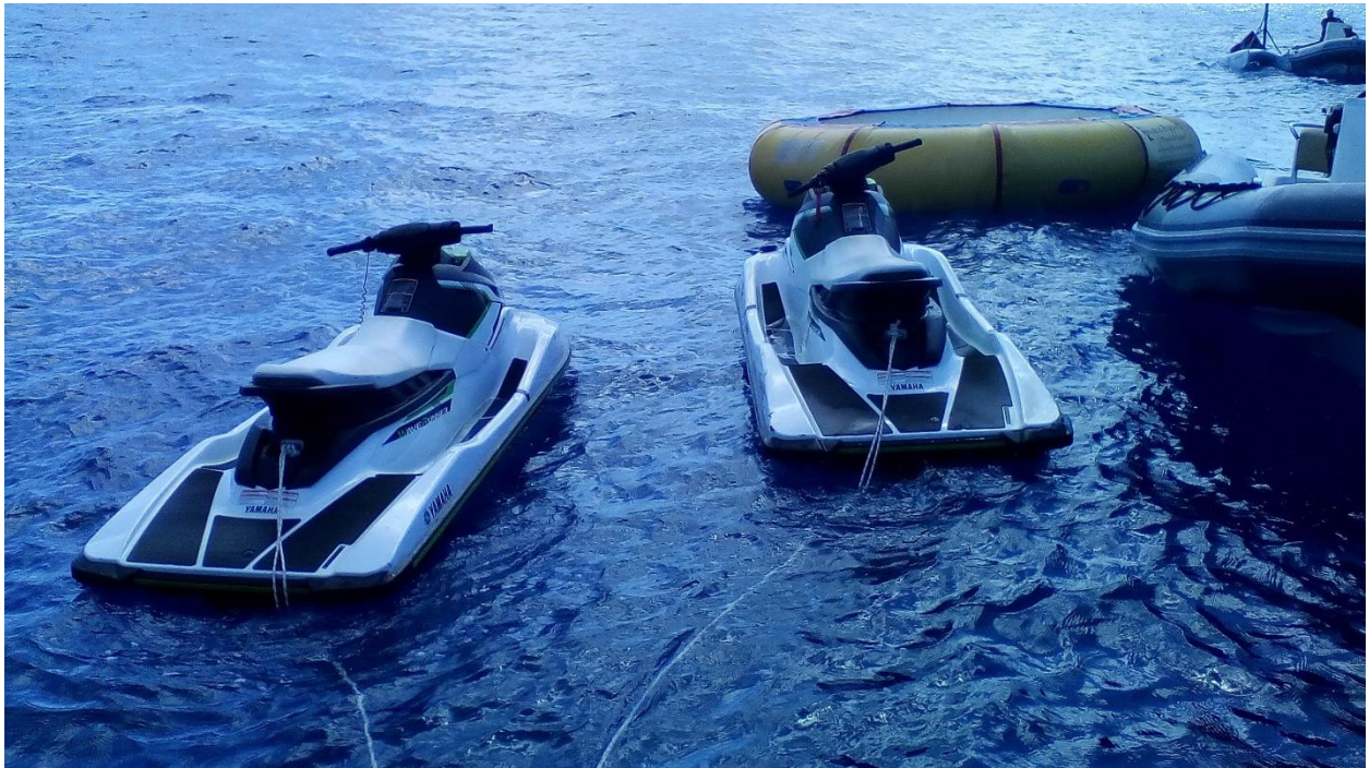
These are 700cc Yamaha Waverunners, with a speed of up to 80km/h on flat water.
